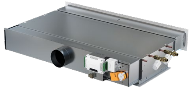
Figure 11. PARAGON AWC, complete with factory-fitted controller, actuator, pressure sensor and valves and valve actuators for cooling and heating water.
