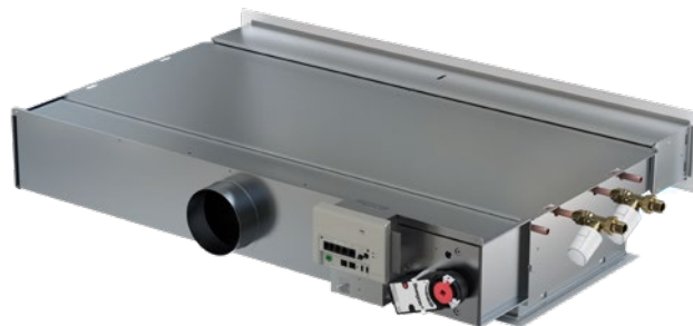
Figure 12. WISE Paragon, complete with factory-installed WISE CU control unit, actuators, and valves and valve actuators for cooling and heating water.
