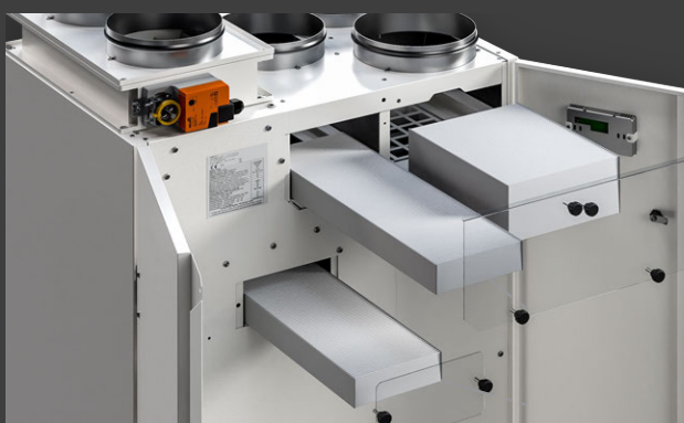
Standard G2 or optional F6 filters, placed in both the supply and intake flow of outside air. Standard filter capacity is ISO Coarse 70% (G2), alternatively an ISO ePM10 60% filter can be installed.
