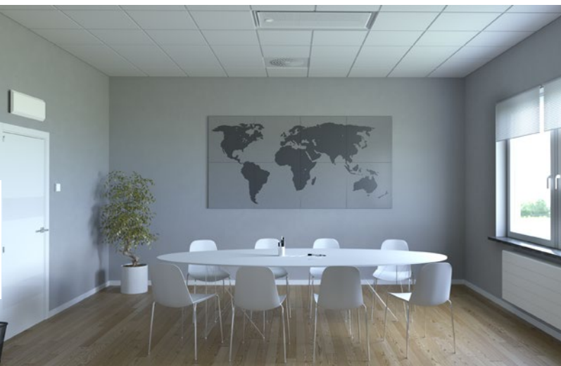
Conference room with setpoint selector switch and demand-controlled air regulation as well as waterborne cooling and control of radiators.
