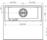
The distance of the grease filter from the edge of the hood is 20 mm.
