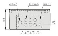
Figure 3. SuperWISE II, SuperWISE II SC underside, measurement figure (mm).
