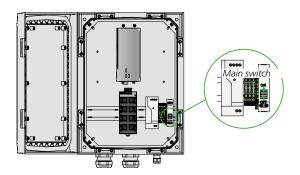
Turn off the power using the main switch before any work is started
