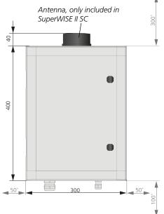
Figure 1. SuperWISE II, SuperWISE II SC, measurement figure (mm). \*Minimum free clearance to nearby installations.
