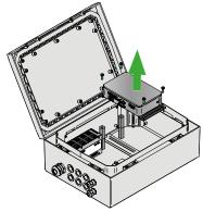
Disconnect all the cables to the control unit, loosen the four screws and lift out the control unit.
