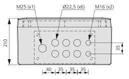
Figure 6. SuperWISE II 2K, SuperWISE II 2K SC underside, measurement figure (mm).
