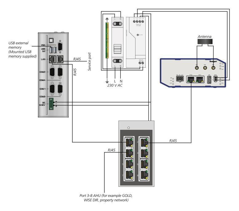
Figure 11. SuperWISE // 2K, SuperWISE // 2K SC, connection.
