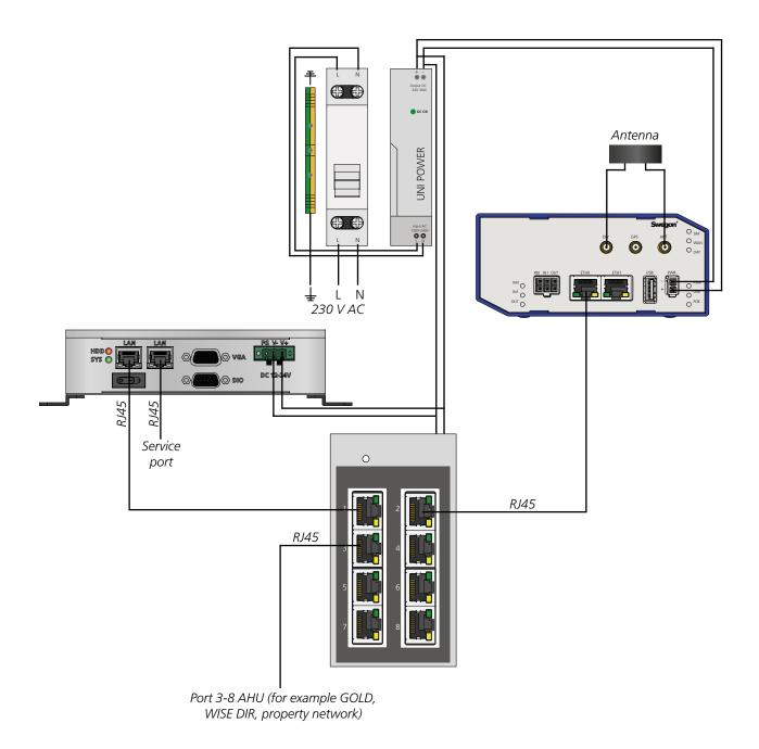
Figure 9. SuperWISE //, SuperWISE // SC, connection.
