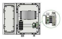
Turn off the power using the main switch before any work is started.
