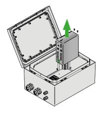
Disconnect all the cables to the control unit, loosen the two screws and lift out the control unit.
