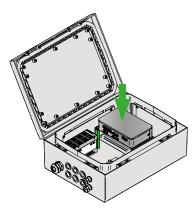
Place the control unit on the 4 spacer bolts and screw back the screws. Reconnect the cables and switch on the power using the main power switch.
