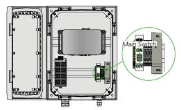
Turn off the power using the main switch before any work is started.
