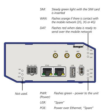
Figure 14. LED key Swegon Connect control unit.
