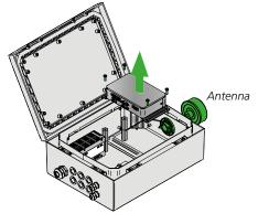
Disconnect all the cables to the control unit, loosen the four screws and lift out the control unit. Fit the antenna in the top of the enclosure and tighten the lock nut on the inside.
