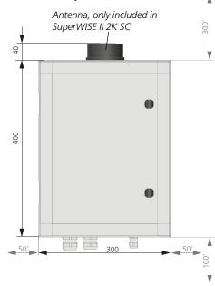
Figure 4. SuperWISE II 2K, SuperWISE II 2K SC, measurement figure (mm).
