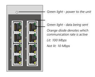
Figure 15. LED key switch.
