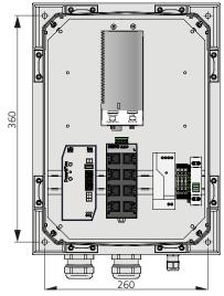
Figure 5. Holes for installation (mm), SuperWISE // 2K, SuperWISE II 2K SC. 4x installation screws (clearance hole  $\emptyset = 8$  mm), screw selection based on the substrate.
