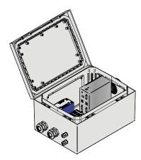
Connect the cables and the antenna. Switch on the power using the main power switch.
