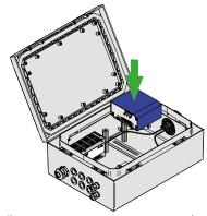
Fit a DIN rail-mount on Swegon Connect and mount on the DIN rail in the bottom of the cabinet. Connect the antenna and cables, see "Connection".
