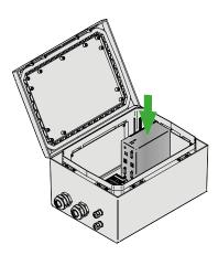
Place the control unit on the bottom of the cabinet and screw back the screws. Reconnect the cables and switch on the power using the main power switch.
