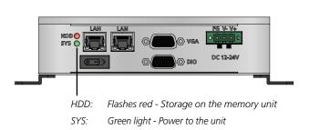
Figure 12. LED key SuperWISE II control unit.
