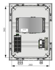
Figure 2. Holes for installation (mm), SuperWISE II, SuperWISE II SC. 4x installation screws (clearance hole  $\emptyset = 8$  mm), screw selection based on the substrate.
