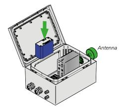
Fit the antenna in the top of the enclosure and tighten the lock nut on the inside. Mount the Swegon Connect on the bottom of the cabinet.
