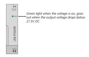
Figure 13. LED key DC power supply.
