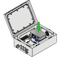
Refit the control unit and connect the cables. Switch on the power using the main power switch.
