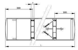
Figure 10. Connection -I, top view. a = adjustment allowance suspension fittings 43 mm.
