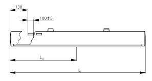
Figure 9. Connection -I, side view. L = length FRB Lu = length of lower section's subdivision
