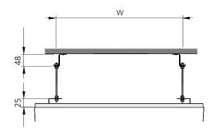
Figure 11. Assembly fittings SYST MS. FRB: W = 326 mm
