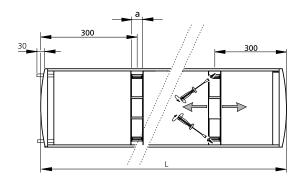
Figure 8. Horizontal connection at the end -H, top view.  $a = adjustment \ allowance \ suspension \ fittings \ 43 \ mm.$
