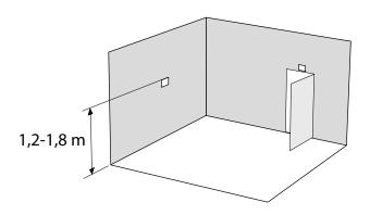
Figure 1. Placement of WISE OCS on the wall.
