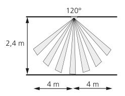
Figure 3. Detection range, ceiling mounted.
