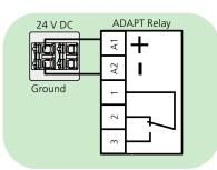
Connection of relay for connection of additional actuators
