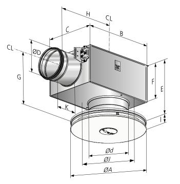
Figure 1. WISE Sphere C, dimensional figure.
