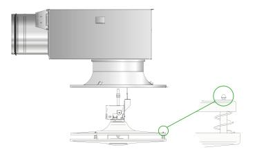
When refitting, fit the pin in the hole in the cone, press the diffuser face upwards at the same time as the knob is slid back.
