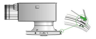
Locate the knob that protrudes from the diffuser face, slide the knob along the slot, the diffuser face is loose at the end position.
