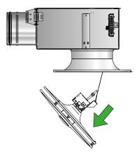
Open diffuser front, disconnect the measuring tubes and cables from WISE CU.
