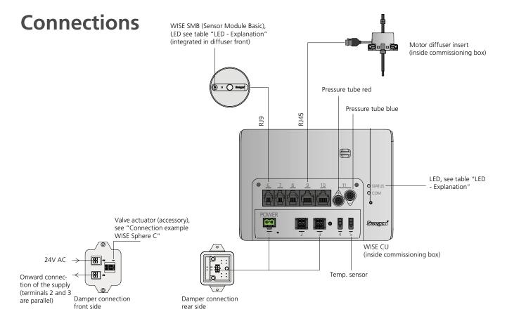
Figure 3. WISE Sphere C, connection.
