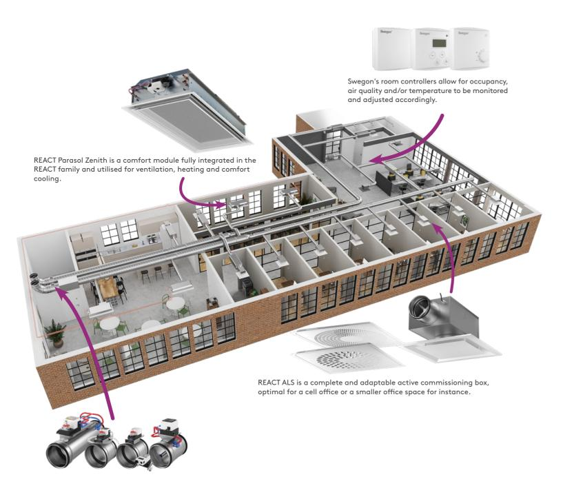
The duct mounted products in the REACT family manages variable air flow, constant air flow, pressure control, pressure measurement, air flow measurement as well as combinations of these.
