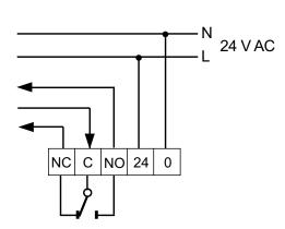
Figure 6. Wiring diagram. NC-C is closed if no occupant is present; NO-C is closed if an occupant is present.
