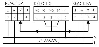
Figure 9. Wiring diagram for a variable flow damper with simplified operation, min. or max. airflow. For more functions, see the installation instructions for each specific VAV damper. The wiring diagram applies only to the REACT controller.
