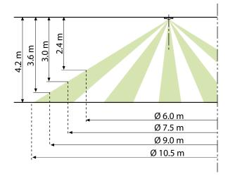
Figure 5. Detection zone. Ceiling-mounted DETECT O T360.
