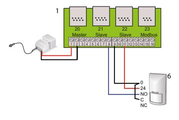
Figure 7. Wiring diagram for ADAPT Damper.
