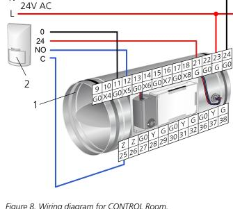
Figure 8. Wiring diagram for CONTROL Room. 1 = CONTROL Room for room regulation 2 = DETECT O
